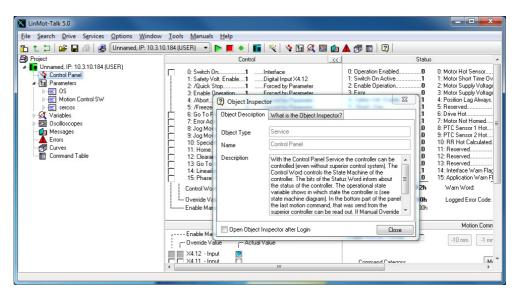
The Object Inspector window can be dragged away or closed. It can be reopened with F1.
