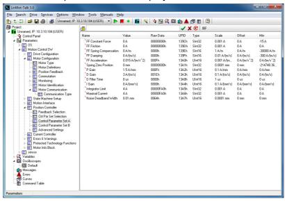
Parameters, which are marked as live ( ), can be altered while the drive's firmware is running; other parameters can only be changed when the software is stopped.
