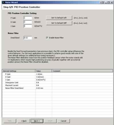
It is recommendable to start with the default soft settings, because the parameters can be changed any time later on (by restarting the motor wizard or by setting in the parameter tree directly).
