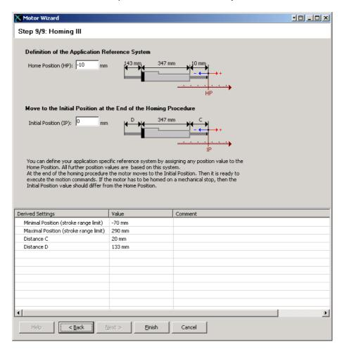
At the end, press finish. If the firmware on the drive is still running, an appropriate message will be shown. All parameters will now being written to the drive.
