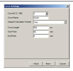
Set curve ID to 3, Curve Name to "SineIn", Curve Length to 500ms, Start Point to 50mm and End Point to 0mm. Click twice "Next" and then "Finish". Now we have defined the two curve segments and will join them together. Select the two curves
