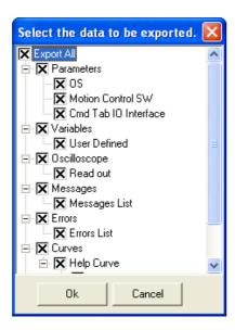
It is recommended to export all. For a configuration recovery it is necessary to select the parameters, curves and command table.
