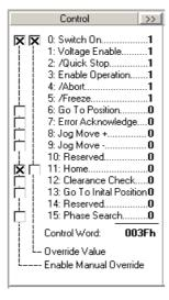
Now turn off and turn on again the "Switch On" flag, this is because of the auto start prevention. At this time, the motor will be powered and position controlled at the actual position. Set the "Home" flag and the motor will initialize against the inner hard stop.
