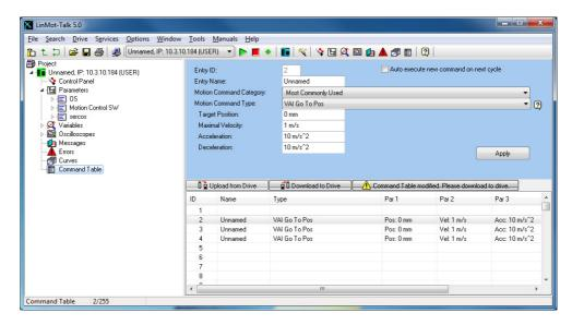
A big variety of commands can be set in this tables, such as motion commands, conditions, sequence directives, parameter access, ... This makes the CT to very powerful functional unit. The CT entries can be accessed (executed) via digital inputs (on X6) or via interface software. The CT tool has the following editing elements:
