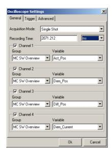
Then press Ok and start the oscilloscope with . The recorded data on will be read out from the drive and displayed, which will look somehow like the following.
