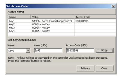
A maximum of four keys can be set on the drive. Under Active Keys all valid installed keys are listed (key value and access code).
