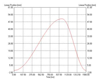
Now the curves must be downloaded to the drive. Therefore press the "Show Curves" button and then the "Download Curves into Drive" button Download into Controller. Then a warning comes up which has to be confirmed and the progress window will display the actions taken to download the curves.
