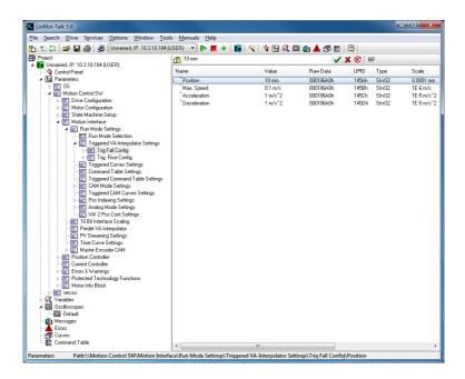
This is all we have to configure. The speed, acceleration and deceleration can also be defined at this place in the parameter tree. The motor can now be started the same way as described under 3.13 Control Status.
