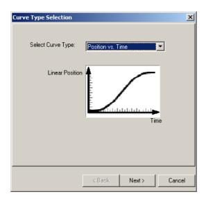
As we want to define a curve in position vs. time mode we can keep the default selection and press the next button.
